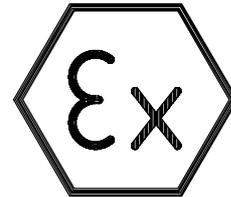
Since 1st July 2003 devices and components only, which meet the requirements of the European Regulation 94/9/EG, may be used in explosion - hazardous areas. Consequently non - electric devices used in explosion - hazardous zones must be checked for their conformity with the current regulations, too.
